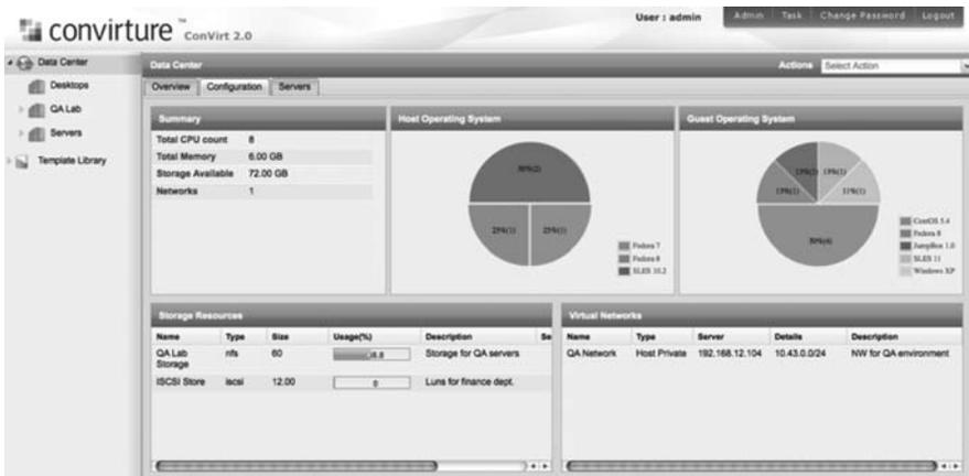
Figure 7.4 ConVirt 2.0 Centralized Monitor for Xen and KVM. The data center-level configuration view provides detailed information about operating systems, storage, and networks resources in your environment. (Licensed under the GNU Free Documentation License.)
