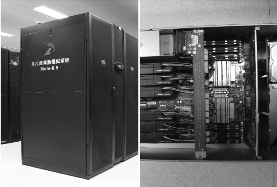
**Figure 3.4** Left: The Mole-8.5 Cluster at the Institute of Process Engineering in Beijing. It consists of 372 nodes, most with 6 Fermi Tesla C2050 GPUs. Right: single node of Mole-8.5 system (courtesy of IPE, photos by Xianfeng He).
