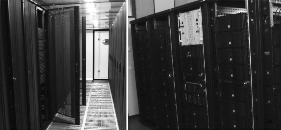
**Figure 3.1** Left: NAOC GPU cluster in Beijing, 85 nodes with 170 NVIDIA Tesla C1060 GPUs, 170-teraflop hardware peak speed, installed in 2010. Right: Frontier Kolob cluster at ZITI Mannheim, 40 nodes with 40 NVIDIA Tesla C870 GPU accelerators, 17-teraflop hardware peak speed, installed in 2008.
